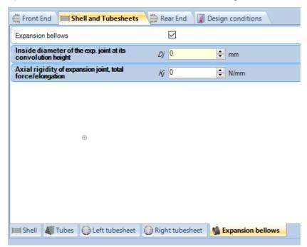
After running the wizard and creating the exchanger, the properties of the joint will be visible in the shell tab. It is also possible to add them directly to the shell after running the wizard, if they have not already been entered previously.
