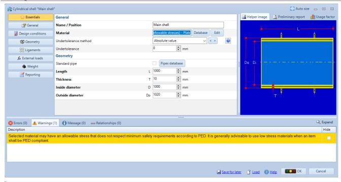
Selected material may have an allowable stress that does not respect minimum safety requirements according to PED. It is generally advisable to use low stress materials when an item shall be PED compliant.
