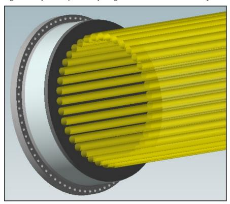
The tube bundle of this vessel is defined with 180 tubes: only the outer ring of tubes is rendered, which shows the user the overall footprint and allows easy selection for modification. Drawing the inner tubes would create a heavier model without any real benefit for the purpose of NextGen.
