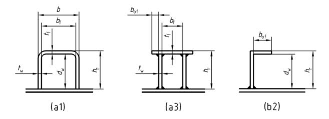
Some of the possible reinforcement configurations for rectangular vessels
